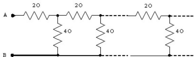
The equivalent resistance between the point A and B is
